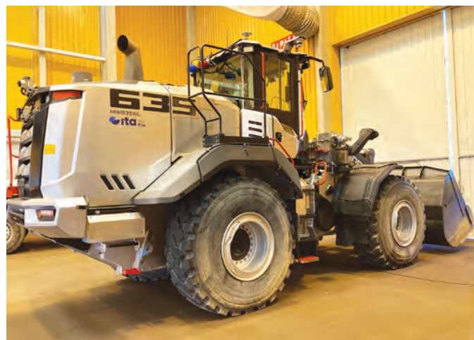
ABOVE: The autonomous wheel loader can be monitored and controlled remotely via teleoperation, with the operator maintaining full oversight.
