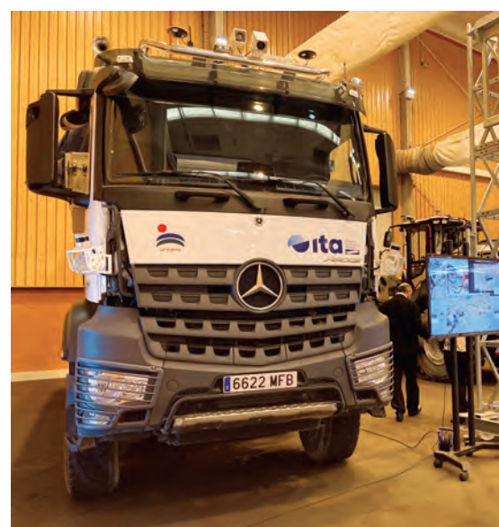
The autonomous dump truck can work alongside other machines and equipment during aggregate transport, significantly improving operational efficiency.
