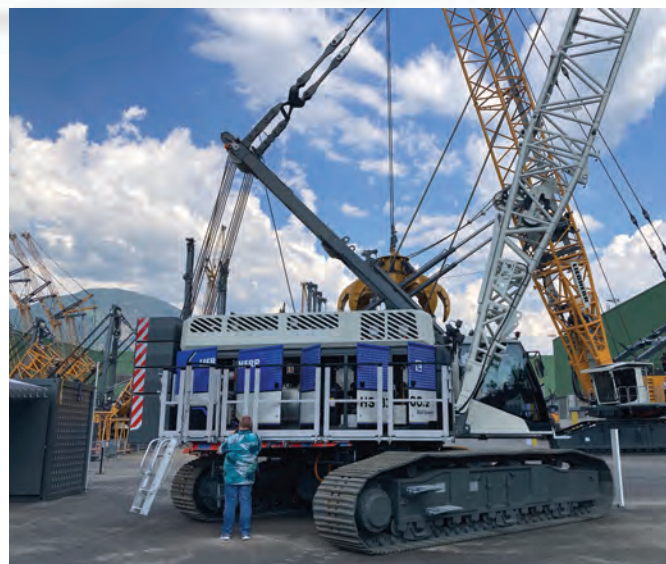
ABOVE AND LEFT: The HS 8100.2 dual power is seen here at the Liebherr Nenzing facility. All main components of the machine are electric: travelling gear, swing drive, luffing winch and free-fall winches.
