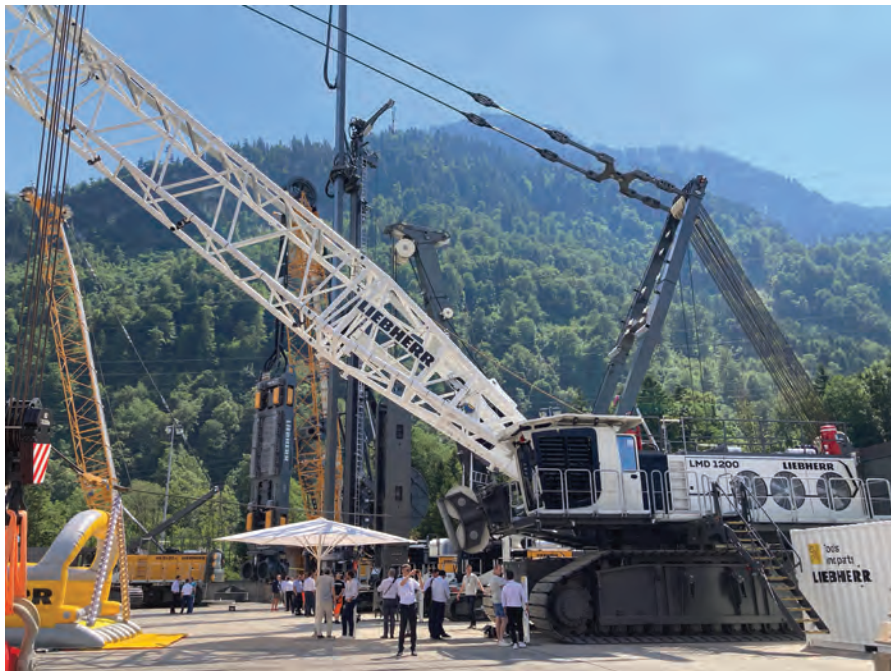
ABOVE: The new LMD 1200 dragline machine on display at Liebherr Nenzing's 50th anniversary event. Available globally, it is suitable for both wet and dry mining applications.
