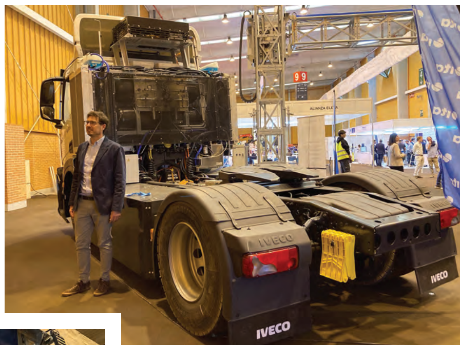
The EH2T truck incorporates an electric motor that delivers the same performance as the original diesel engine, ensuring there is no loss of operating performance. The vehicle now serves as a mobile laboratory for ITA and will be used to collaborate with industry stakeholders.
