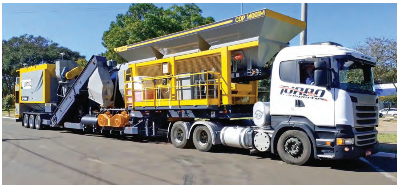
The mobile Lintec CDP1400M asphalt mixing plant powers Mexico's road modernisation, delivering high-output performance with up to 15% reclaimed asphalt pavement (RAP) for greener, more cost-effective construction.
