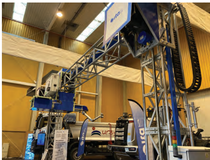
In another project, ITA has been working on a robotic 3D printer for refurbishing and customising facades.
