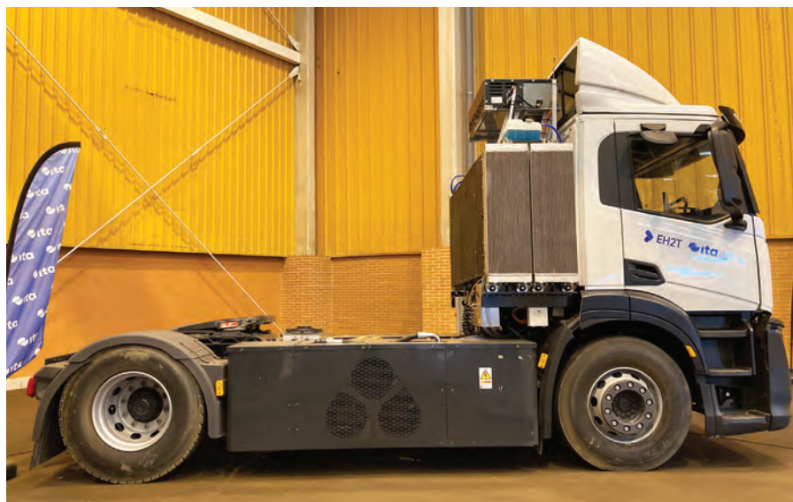
ITA's EH2T project involved retrofitting a 40-t diesel truck to provide a more sustainable alternative. It was first electrified, and subsequently fuel cells and auxiliary systems were integrated. This 'hybrid' truck has been successfully tested on a national road in Spain.
