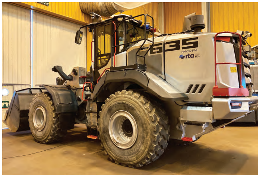
ITA has developed an autonomous wheel loader in collaboration with Turkish manufacturer Hidromek. Still a prototype, the machine is designed for operations in tunnels and hazardous environments, such as demolition sites where dust levels are high and visibility is low.
